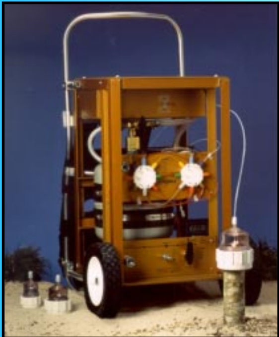
The complete HPFM-C system is field portable with detachable wheels and backpack.
