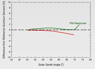
Mean cosine response of seven Apogee SQ-500 quantum sensors. Cosine response measurements were made on the rooftop of the Apogee building in Logan, UT. Cosine response was calculated as the relative difference of SQ-500 quantum sensors from the mean of replicate reference quantum sensors (LI-COR models LI-190 and LI-190R, Kipp & Zonen model PQS 1). The red data are AM measurements; the green data are PM measurements.
