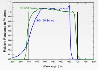
Mean spectral response measurements of six replicate Apogee SQ-100 and SQ-500 series quantum sensors. Spectral response measurements were made at 10 nm increments across a wavelength range of 300 to 800 nm in a monochromator with an attached electric light source. Measured spectral data from each quantum sensor were normalized by the measured spectral response of the monochromator/electric light combination, which was measured with a spectroradiometer.
